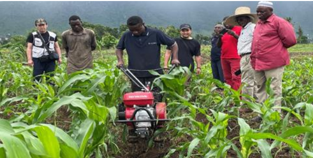
Tiller (FQ650) working inter-tillage in maize fields.
