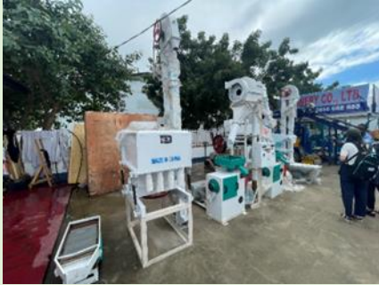
Name/Model: Rice milling plant /TSMJ-20 (1,200kg/h)
