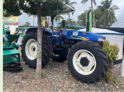
Name/Model: Tractor (NewHolland)/TT75(75PS/4WD)
